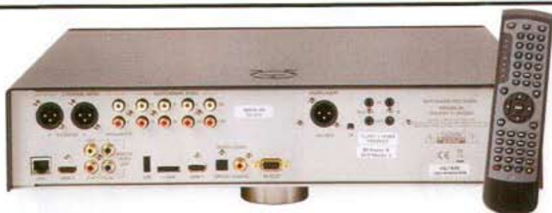
ABOVE: Left to right – ethernet and secondary HDMI ports, component/composite video, USB and e-Sata connections, primary HDMI out, opt/coax digital audio and (above) 7.1 channel plus stereo RCA and balanced XLR analogue audio outs
